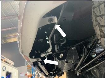
2. Remove four retaining bolts on the underside of the bumper.
