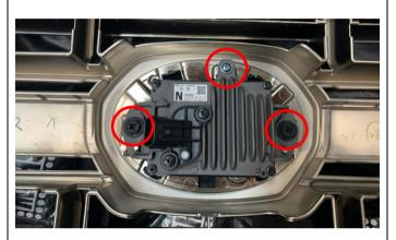
15. Place the grille face down on a soft surface, remove radar using a Phillips head screwdriver and place in a safe spot
