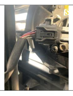
14. Pull the grille forward and unplug the radar module located behind the Toyota badge.
