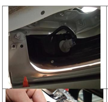
18. Remove the vehicle's plastic indicator access covers (RH & LH), located underneath the indicators to reveal indicator plug.
