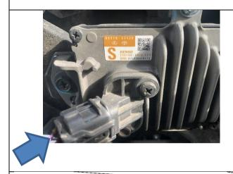
51. Connect radar extension loom to radar module.
