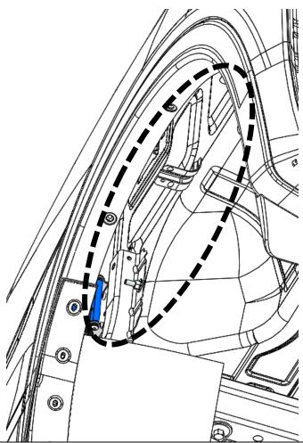
6. Pull the wheel arch liner away and down from the wheel arch flare to gain access between the tub and outside of vehicle.
