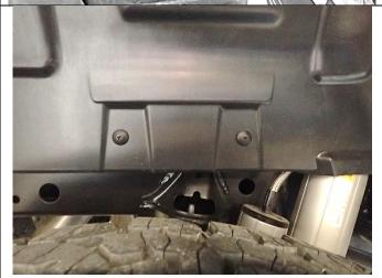
4. Remove four scrivets from the rear RHS wheel arch liner.
