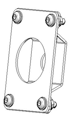
35. Feed the hose through the body and mount, then using LOCTITE THREAD SEALANT 569 tighten the hose to the air chuck.
