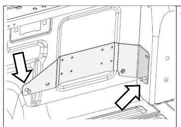
16. Using two M8 hex bolts, attach the support bracket to the OE tie down mounts.
