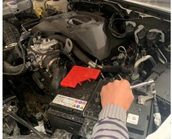
37. Disconnect the negative battery terminal from the battery.
