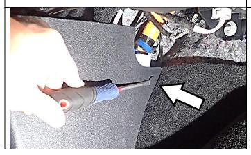
68. From inside the vehicle left hand side, to the left of the foot well, find and remove the christmas tree plug as shown.
