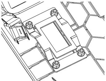
85. Use the four M4 Button head screws to locate the cover plate and switch mount, then tighten using the four M4 washers and four M4 Nyloc nuts.
