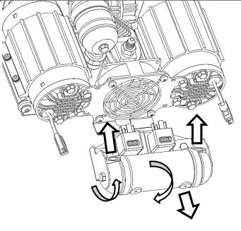
13. Loosen the bolts on the manifold brackets and orientate the manifold body and cap outlets to the directions shown.
