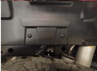
102. Refit the RHS wheel arch liner using the scrivets removed in Steps 4 and 5.
