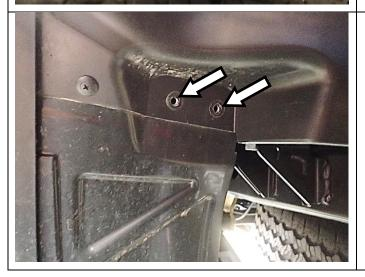
103. Install the provided pop rivets and two M6x18x3 flat washers into the locations of the removed pop rivets from Steps 2 and 3.
