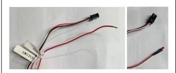
64. Tie back and cover with tape the 'SWITCH CONNECTOR' and wire 'IGNITION SOURCE'.
