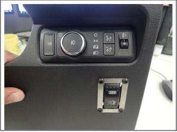
86. Locate the ARB rocker switch supplied with this compressor kit and click into place.
