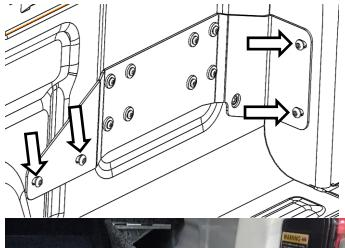
33. Fit four M8 Button head fasteners and tighten to spec.
