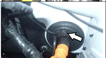
71. Locate firewall grommet located behind the passenger side fuse box.
