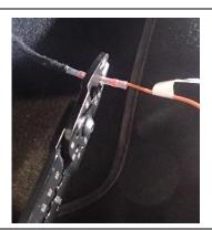
75. Behind the door sill panel, identify the crimp joiner supplied in the ARB harness kit. With a crimping tool, join the vehicle wire labelled "RUN START" with the harness wire labelled 'IGNITION SOURCE'.
