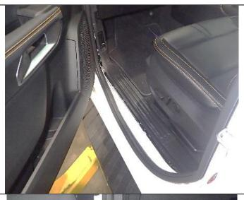
69. Lift and remove the rubber seal surrounding the left hand side sill panel.
