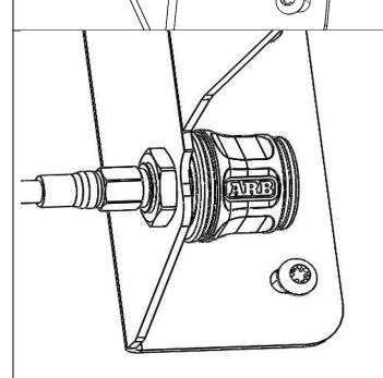
24. Feed the hose back into the hole and tighten the retaining nut for the air chuck.
