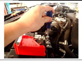
97. On positive battery terminal, remove one of the terminal nuts.
