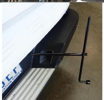
52. Remove vehicle spare tyre from beneath the vehicle tray.
