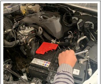
104. Reinstall the battery negative terminal.
