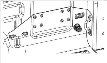
25. Using the original four M8 Button head fasteners, attach the OE tie down points to the side and rear.
