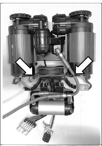
14. Fit 500mm braided hose incl. with the compressor and fittings to manifold.
