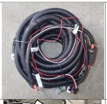
38. Locate the harness trunk with connectors labelled 'COMPRESSORS', 'GROUND' & 'UPFITTER SOURCE'.
