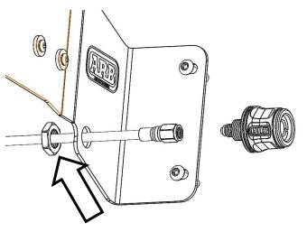
22. Remove the nut from the air chuck and place over the air hose inside the rear guard. Feed the hose through the hole in the body and mounting bracket.
