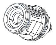
23. Using LOCTITE THREAD SEALANT 569, tighten the air chuck onto the hose.
