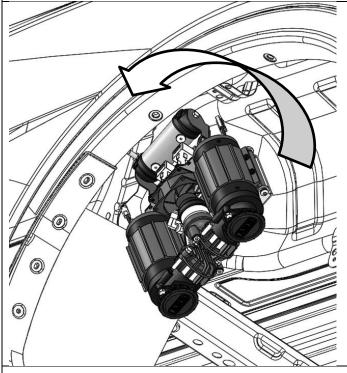
17. To fit compressor, insert into the fitting cavity with the manifold facing up and filters facing down as shown.
