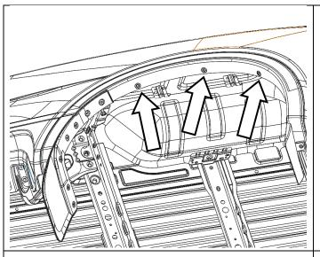
5. Remove the three scrivets from the wheel flare as shown.
