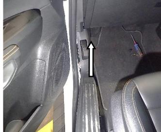
70. Remove door sill panel as shown. This can be removed by lifting the sill panel and then rotating up.
