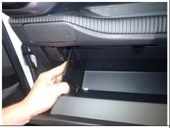
76. Remove vehicle glove compartment.
