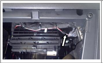
91. On the passenger side of the vehicle, connect the ARB universal switch connector into harness connector labelled 'SWITCH CONNECTOR'.
