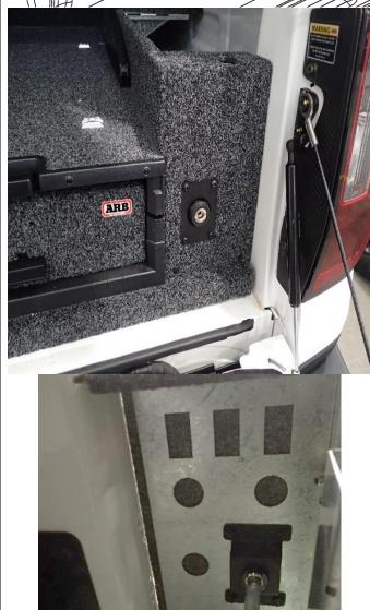
36. At this point, the harness can be installed. Please study the layout of this harness (Part #6821428) and the connectors as these will be referenced throughout the harness install procedure.
