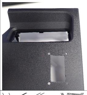
84. Using a multi tool, cut out the scribed area and deburr all the edges.
