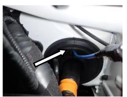
72. With a sharp blade, cut and remove the nipple from the firewall grommet.
