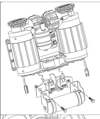
12. Fit the manifold to the compressor assembly using two M6x25 screws and M6 Nylocs included in the manifold kit.
