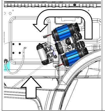
18. Once compressor is inserted rotate the compressor anti-clockwise and gently lower into position.
