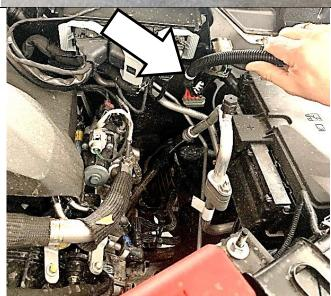
40. Supplied in the accessories bag is a stud mount cable tie. Connect this cable tie to the harness and push onto the stud protruding from the firewall.
