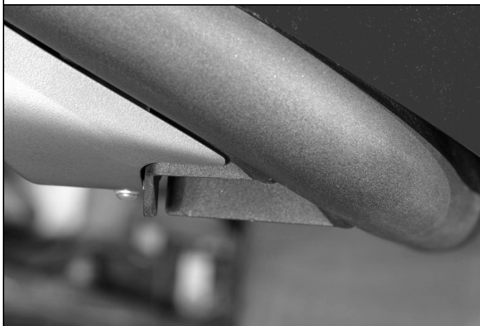
HIGH LIFT JACK LOCATION - CORNER OF RSTB
