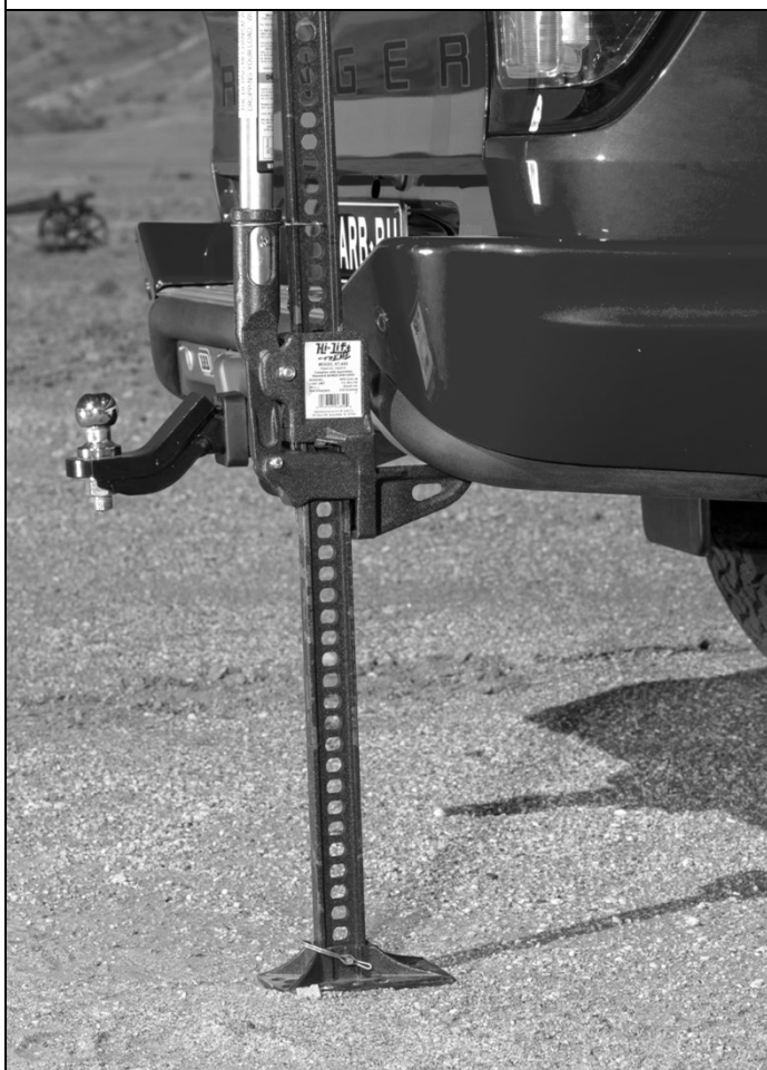
HIGH LIFT JACK LOCATION - CORNER OF RSTB
