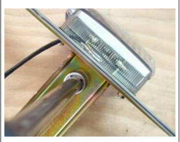
Tighten using 17mm socket. (Viewed from underneath.)
