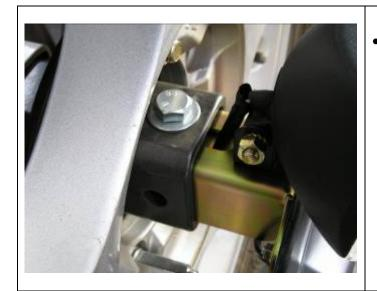
When adjusting number plate bracket, be careful not to cut through loom.
