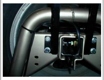
• Cable tie loom to wheel carrier frame.
