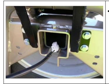
Fit loom through centre of wheel mount as shown. (Viewed from rear of wheel carrier.)
