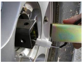
Connect loom to light as shown and fit number plate bracket to wheel mount.
