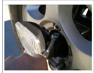
• Tighten M12 bolt using 18mm spanner.
