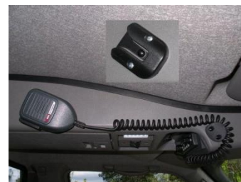
Install microphone clip on acute angle
