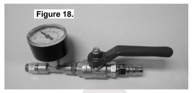
If a leak is found to be present, spray a soap and water mixture onto the bulkhead air fitting. Bubbles should appear at any leak points.
