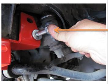
8. Fit the lower rear steering idler bolt & flat washer (*M12 x 120 - Class 10.9*) into place as shown.
