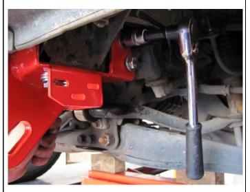
16. Torque the two rear bolts (*M12 x 120 – Class 10.9*) to 109 Nm (*81 lbft*).
