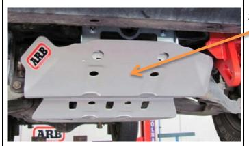
22. Refit ARB Under Body Protection in reverse order to removal in *step 1*.
