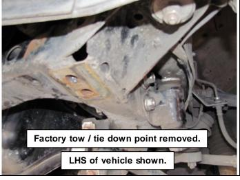
2. Remove the front left factory tow / tie down point.
