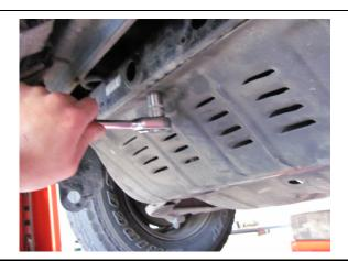
1. Remove stone shield or under body protection.
