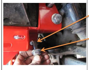
12. Place one *M12 x 1.5 x 40 mm* bolt with a flat washer\* fitted through the recovery point and the hanger bracket.
