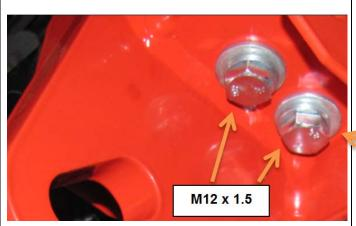
7. While holding the recovery point firmly against the chassis, finger tighten an M12 x 1.5 x 40 mm bolt, spring washer & flat washer\* in to the two remaining holes on the bottom of the chassis.
