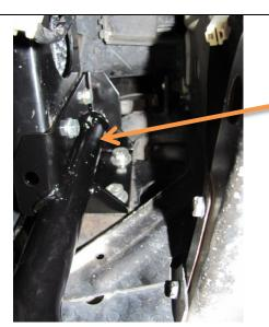
25. Bolt the upper brackets of the bullbar to chassis brace in reverse order to removal using the same nuts and bolts as removed in step 3.
