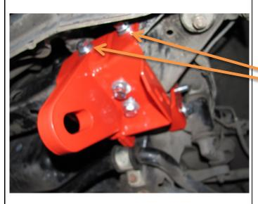
Finger tighten M12 x 1.5 x 40 mm bolts, spring & flat washers in to both holes in the front of the chassis as shown.
