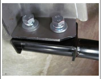
26. Bolt the lower bracket to the recovery point using *M10 x 1.5 x 30 mm* bolts, spring & flat washer.
