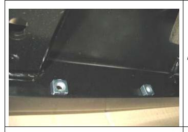
48. Working within the bull bar, insert 2 x M6 caged nuts to inside front face of top pan.
