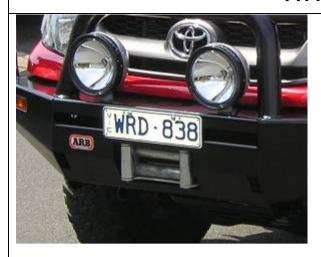
78. Fit number plate to bar using 2 X M6 x 20 bolts, spring washers and standard flat washers. (Winch version shown)
