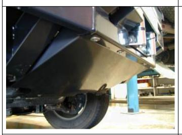
74. Fit the centre stone guard as shown using M8 black bolts, black M8 flat washers, black M8 spring washers & cage nuts.
