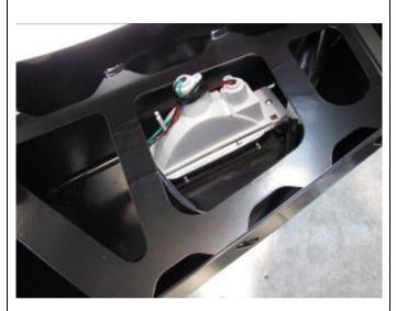
50. Remove the fastening screws and nuts supplied with the turn signal/clearance lamps and replace these with the four screws provided in the kit. Push the square plastic plugs into the holes on the turn signal bracket. Fasten the turn signal lamps to the bull bar as shown.
