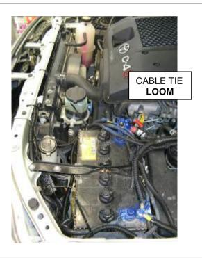
47. Using the cable ties supplied, secure the loom keeping clear of any hot, sharp or moving surfaces.
