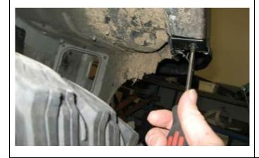
18. Fit a plastite screw to secure the rear of the flaret as shown
