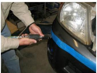
NOTE: If fog lamps are fitted, disconnect them. Check that there is nothing behind the bumper such as wiring in the cutting path before proceeding
