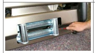
61. Fit roller fairlead into cutout and refit bolts and tighten firmly.
