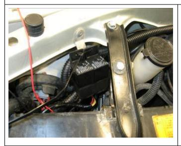
44. Find a suitable place and mount the relay.
