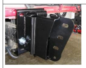
65. Loosely bolt the impact absorbers to the chassis using the factory studs with the large M10 flat washers, spring washers and M10 x 1.25 fine pitch nuts.
