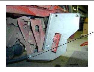
20.Fit 12mm hardware to where indicated in photo, making sure to use large 40mm x 12mm offset washer to cover hole on inside of rear mount. Pre 05 model shown.
