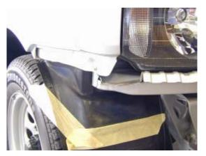
22. Before fitting bar to vehicle, cut plastic inner guard to approximately the top line of masking tape in photo on left. Alternatively the inner guard can be removed totally.
