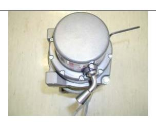
3. To place the clutch handle in the correct position, the winch gearbox must be rotated 72 degrees (2 hole spacings) in a clockwise direction when viewed from gearbox end. Place the winch on its end and remove all gearbox bolts. Gently raise the gearbox just enough to rotate it. When the correct position is located, refit all bolts and tighten.
