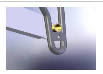
21. On 05 onwards vehicles place spacer tube in tie down point as shown. Secure using M12 X 40 mm bolt, spring washer, off-set washer and nut placing the off-set washer on outside surface against tie down.
