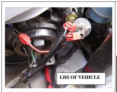
46.Pull indicator loom up into engine bay to scotch lok wiring onto vehicle indicator/clearance lamps
