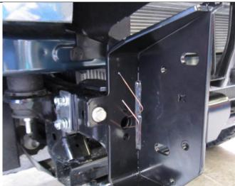
46. Re-use one of the chassis bolts, removed at step 15, to firmly locate the bull-bar mount bracket to the chassis.
