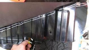
73. Remove the two wing stone guards and mark a second line 5mm above the first line on the RH and LH wheel liners.
