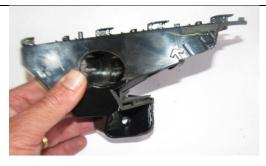
34. Use a hack saw to cut the RH and LH bumper retaining brackets. Once these cuts have been completed the parts should look like the adjacent images.
