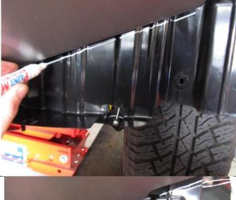
72. Loosely fit the RH and LH wing stone guards to the bull-bar. As shown on the adjacent photo, use a white marker to draw a line on the wheel liner at the lower rear edges of the stone guards.
