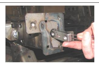
44. Insert the nut plate, from the bull-bar fitting kit, through the front flange of the chassis rail with the wire attached.
