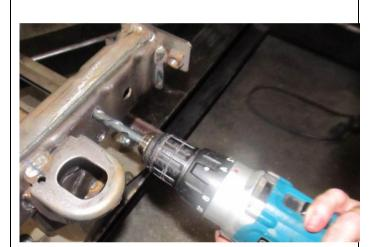
42. Replace the Ø13mm drill bit with a Ø10.5mm drill bit and pass the drill through the Ø13mm holes.
