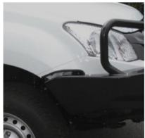
Position the bar so that the rear of the wing is parallel with the vehicle fender and lines up with the wheel arch. The nominal distance between the vehicle fender and the bull-bar is 48mm.
