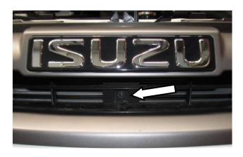
5. Remove and retain the front screw holding the bumper grill in place.
