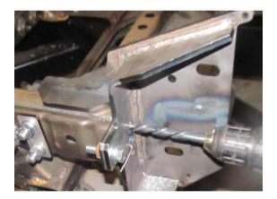
47. Use a punch to mark the two holes in the front of the chassis rail.
