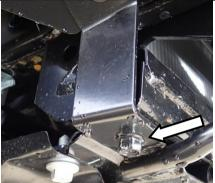
71. Fit the 2 wing stone retaining brackets to the vehicle chassis using the outer bolts holding the vehicle recovery points.
