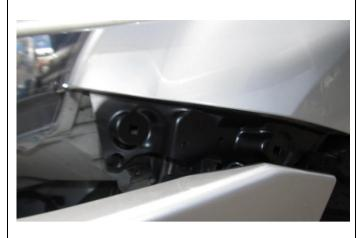
36. Remove the bumper and mask the vehicle fenders and headlights. Use a spray can to paint the region immediately below that RH & LH vehicle fenders black.
