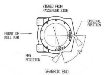
NOTE: Take care not to lift the assembly more than a couple of millimetres while rotating to the desired position to avoid unmeshing the gears.
