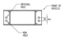
2. New mounting holes must be drilled in the roller fairlead in order to line up with the winch mounting holes in the bull bar. (Refer to diagram 1.)
