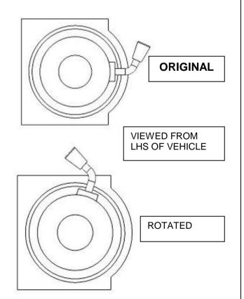
Note To fit an 8/9/9.5/000lb warn winch, rotate gearbox 72° counter clockwise.
