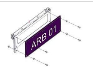
28. Using 4 SS M6 button head screws, SS M6 washers and M6 flange nuts attach the number plate to the pivot bracket.
