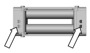
9. Drill 2 new Ø13mm holes in the roller fairlead (RFL) supplied with the winch **20mm** below the OE holes as shown.
