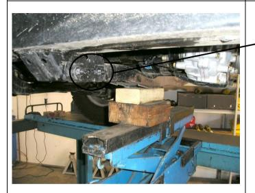
Working on one side at a time, support the gearbox cross member and remove the two outer bolts. Discard the bolts.
