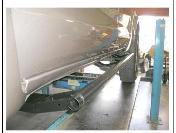
12. Align the side rails to the vehicle and tighten all the bolts.
