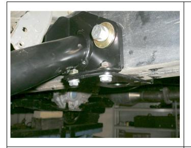
11.Using two M8 x 20mm bolts, M8 flat washers and M8 flange nuts, secure the clamp to the centre support tube.
