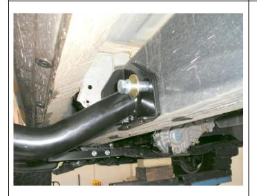
10.Using a ½" x 4 ½" bolt, ½" spring and flat washer and a sleeve, join the centre mount to the clamp bracket.
