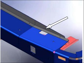
Carefully place the top plate onto bar and attach to front holes using M6 stainless button head cap screws.
