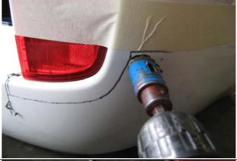
9. For a neater finish use a 25mm hole saw to cut the edges as shown in the picture.
