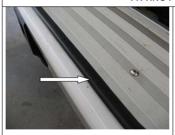
21. Place rubber extrusion around aluminium plate as shown. Trim edges flush and attach to bar using M6 stainless button head cap screws.
