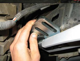
16. Working on one side at a time remove bolts and place the 8mm packers between bar mount and chassis then tighten.
