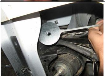
19. Place the M12 cage nuts into cage nut plates and insert through hole in the side of the chassis. Attach to bar using M12 bolts, spring washers and flat washers. Tighten all bolts. Once the height has been set, and bar wing level with bumper cut, tighten all bolts.
