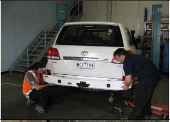
15. With the help of another person place bar gently on vehicle and secure loosely with original tie down bolts in chassis.
