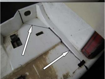
8. Mark a line on top surface of bar as per the picture and join up to the line marked in step 7. Remove the fog light and place aside.
