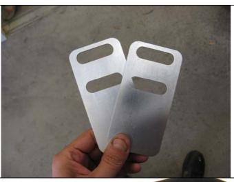
18. Make sure the distance is no less than 10mm. If not add the 3mm packers to achieve a minimum 10mm. NOTE:
