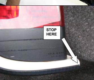
12. Apply pinch weld to cut surface stopping at the base of the fog light as shown. Fit bumper back on vehicle.
