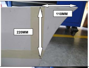
5. From the top front edge of the bumper measure towards the rear 110mm and make a mark. From this point measure down 220mm and mark. This is the cut line.
