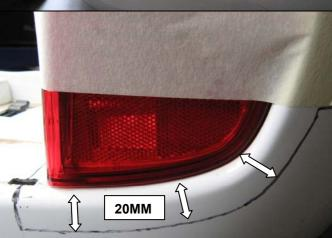
From the edge of the fog light/reflector measure and mark several points 20mm away from the lens. Join these marks to form a line as shown in the photo.
