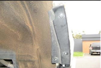
Cut top of original mud flap as shown and attach to vehicle and bumper with original hardware.
