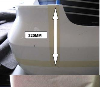
6. From the top edge of the bar measure straight down 320mm and mark. Join marked lines with a length of masking tape making sure it is straight. This will be the cut line. NOTE: Make sure line is straight by sighting down length of bumper. If not re-adjust tape so a straight line is achieved particularly around corner near reflector.
