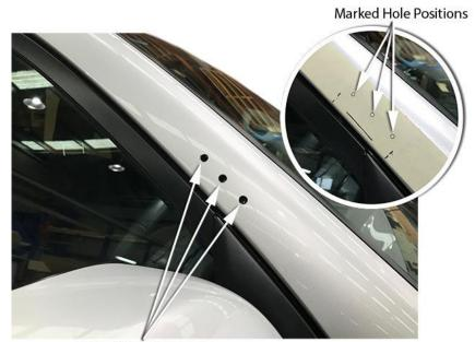
Drilled Holes 8mm Dia
