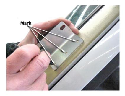
Drill a pilot hole at each of the three (3) marked hole positions.
