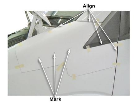
Drill a pilot hole for each of the marked hole positions.
