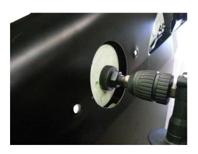
De-burr and paint all holes (earth boss, outer guard and inner guard panels) including the 9.0mm diameter holes.
