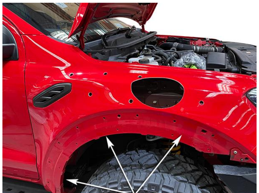
Fender Flare & Inner Guard Liner Removed
