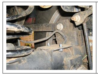
1. Fit 2 M8 x 20 bolts with flat washers to bump stop plate from underside as shown.
