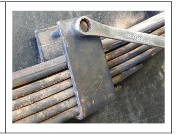
To disassemble the leaf spring ensure the spring is well secured with a clamp before releasing the centre spring bolt as shown. Use vice grips to secure the round head of the centre bolt if required.
