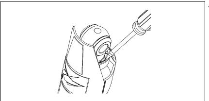
4. Check Retainers are completely secured by Guard. Use a flat blade screwdriver to poke Retainer under tab on guard if required.
