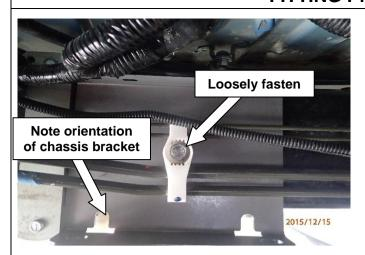
6. Move the fuel lines forward and slide the Chassis Bracket underneath as shown.
