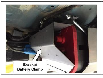
25. Place Bracket Battery Clamp in position onto the Battery Tray.
