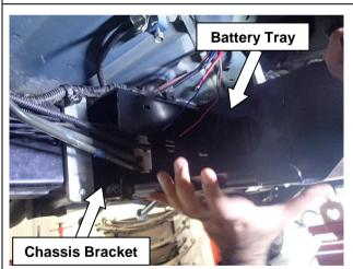
15. Slide Battery Tray over Chassis Bracket and vehicle chassis so that it protrudes on the outboard side of the chassis. Adjust height of tray and ensure it clears vehicle looms and sits flat over chassis.
