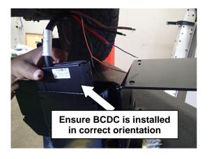
13. Insert BCDC (*not supplied*) into Battery Tray in the direction as shown.
