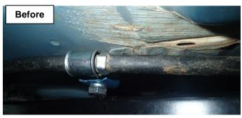
28. Refit the saddle clamp that contains the handbrake cable to the vehicle as shown. Use the Bolt M8 x 20mm supplied with the Battery Tray Kit in place of the factory bolt to fasten the saddle clamp.
