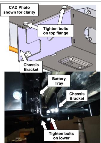
20. Fasten Battery Tray through the 4 slots, each located on the top and lower flanges of the Chassis Bracket using 4X Bolt M8 x 20, 4X Washer Flat M8 and 4X Nut Flange M8. Tighten to specified torque.
