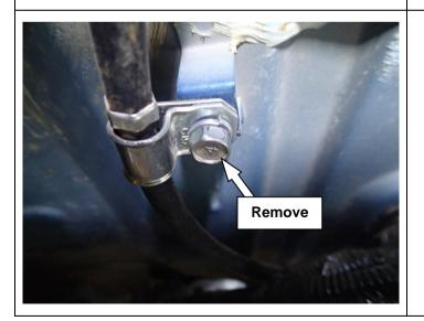
5. Remove the 1X M8 bolt (*retaining the hand brake cable*) from the vehicle body and discard.
