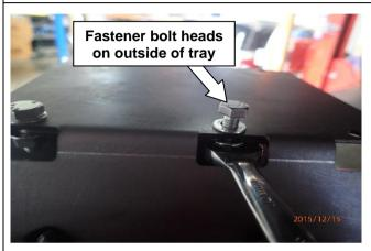
14. Fasten the BCDC (not supplied) to the tray using 4X Bolt M6 x 1.0 x 20, 4X Washer M6 Flat and 4X Nut Flange Hex M6 x 1.0. Tighten to specified torque.
