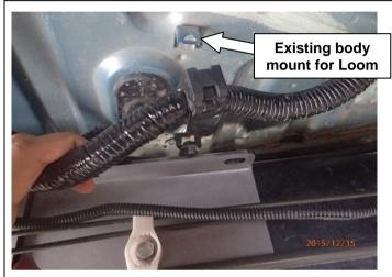
8. Unclip vehicle loom from existing body mount.
