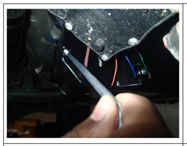
26. Pass in 2X Bolt L M8 x 210mm from rear of battery tray through to holes on Bracket Battery Clamp.
