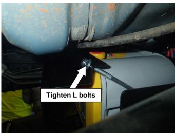
27. Fasten L bolts with 2X Nut Nyloc M8 x 1.25 and 2X Washer Flat M8.
