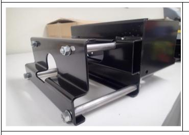
7. Photo depicts assembly of Battery Tray and Clamp out of the vehicle for clarity.
