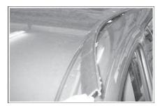
Lift front of the trim from outside edge of roof. Twist outwards to unhook as shown in the diagrams.
