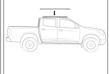
15 Once Pioneer Underbars have been aligned properly, tighten all M8 hardware using 13mm socket wrench or 13mm spanner. Ensure channel nut has rotated within Pioneer underbar and is fixing Pioneer securely.
