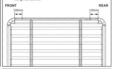
14 After underbars have been correctly fitted, place the Pioneer Platform on top of the Backbone. Align the underbars with the top tabs and ensure the M8 hardware fits into underbar channel.
