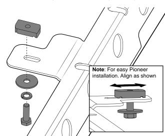
13 Install Pioneer Underbars with slots indicated (42100 REAR: 125mm from Rear (using slots) FRONT: 100mm from Front (drill) The rear slot will have to be drilled with an 8.5mm drill bit. For detailed underbar installation instructions, refer to Pioneer fitting instructions.
