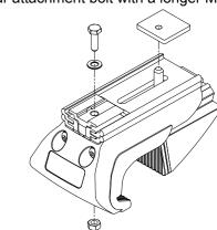
Fitting additional spacers follow the same process as fitting the first two spacers, the first spacer being a type 1 spacer followed by type 2 spacers for however many that are required. For a three leg height spacer system first slide in a type 1 spacer followed by two type 2 spacers.
