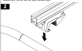
Pull the inner and outer clamp legs together around the rails. Adjust the heavy duty crossbar so that the crossbar over hang is equal both sides, finger tighten the crossbar attachment bolt.
