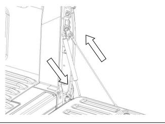
2.3) When complete open and close the tailgate to ensure correct operation. Make sure there is no binding, cables protruding or contact of struts to the vehicle tailgate or body of the vehicle.
