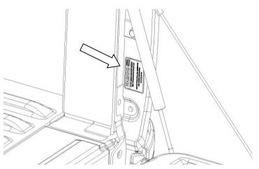
2.4) Fit warning label to vehicle tub as shown in the image. It must be fitted to the larger spring assist side and placed just above the lower tail light mounting screw.
