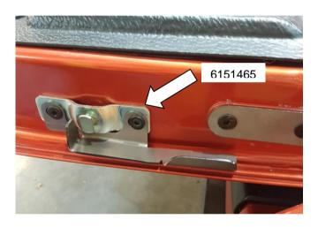
1.4) Remove the bolts from the existing strap mount on the tailgate and discard them. Fit to the cable guide bracket (3750241R) two M8 ultra-thin socket screws (6151465) and mount this over the existing strap mount bracket on the tailgate and leave screws finger tight.
