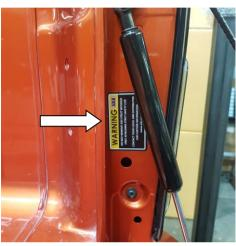
2.3) Fit the warning label (2125702) to vehicle tub as shown in the image.It must be fitted to the larger spring assist side and placed just above the lower tail light screw position.
