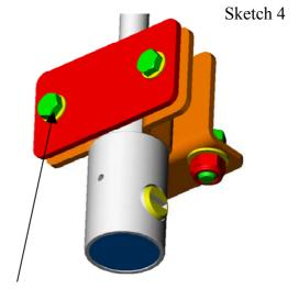
Tighten the M6 screws to 3.5 Nm to secure the cable lock in to the upper bracket.
