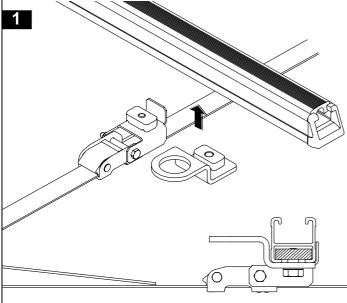
Wrap the snap hook end of the strap over the ladder runs. Snap the hook onto the hook bracket ensuring the safety latch is fully closed onto the hook. Pull the strap to tighten around the ladder rung. Check that the ladder is secure. To release the ladder, press the camlock latch and pull the strap back through the camlock, unhook the snap hook, if travelling with out a ladder, locate the snap hook onto the hook bracket.
