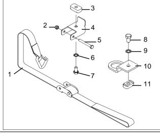
Insert the camlock and hook bracket onto the underside recess of the crossbar. Push the attachment bolt up and turn the bolt so that the channel nut is fully located across the crossbar as per the diagrams. Position the camlock and hook bracket to suit the ladder, tighten the bolts.
