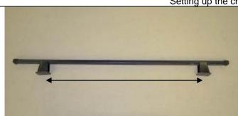
Measure the centre distance between the 25mm holes in the canopy shell.
